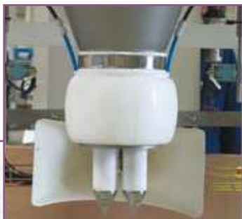
Boca hinchable + doble sonda Inflatable bagging spout + double deaeration rod
